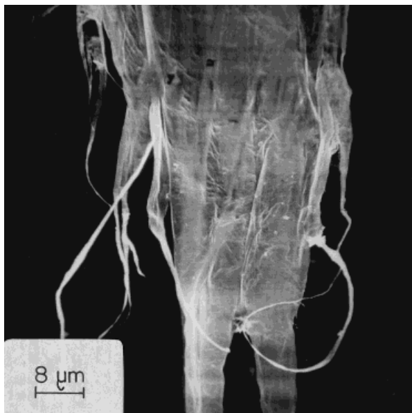
Figure 13 Fractured area of the uncrosslinked GUR 412-PIR blend.
